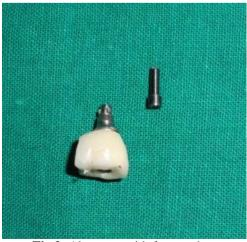
Fig 3: Abutment with fractured screw
